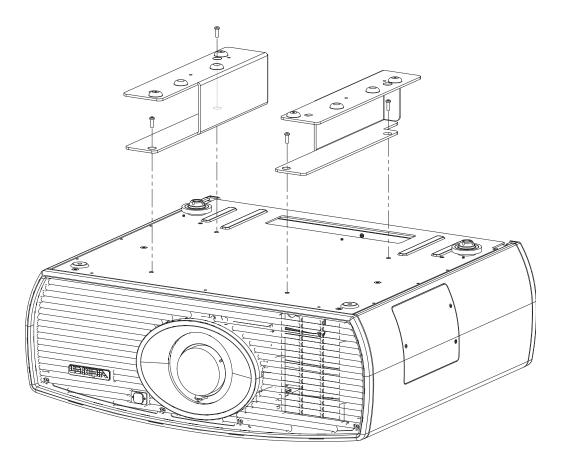
Figure 3-6. Vision 65/75 with Ceiling Mount Adapters/Projector Stands
